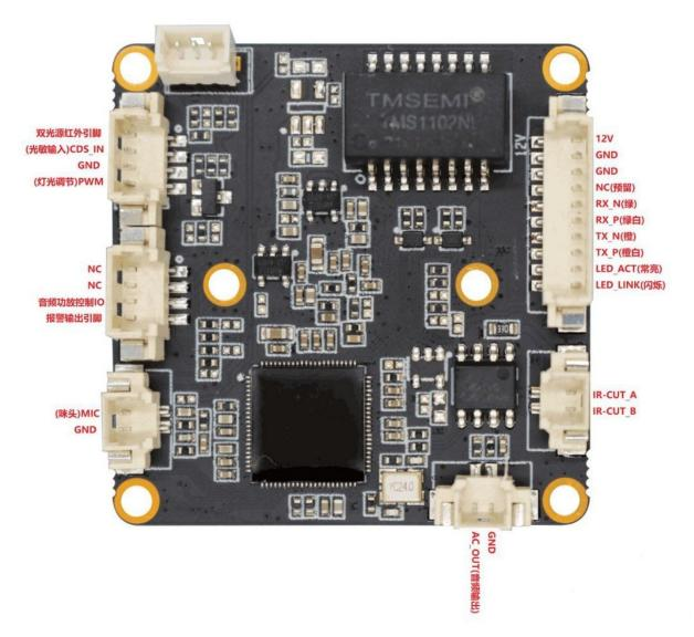
IR-CUT direction Description: IR-cut\_B is + (red), IR-cut\_A is - (black)
